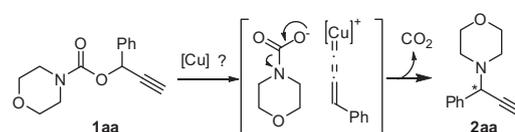
**Scheme 1.** General reaction scheme for Cu-catalyzed asymmetric decarboxylative propargylic amination.
